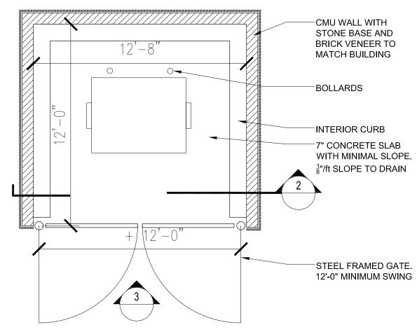
1. TRASH ENCLOSURE PLAN SCALE:1/4"=1'-0"
