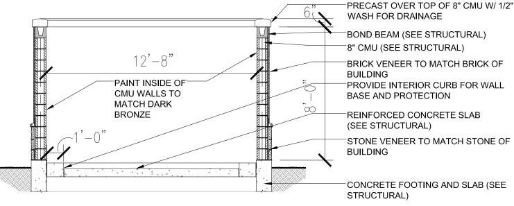
2. TRASH ENCLOSURE SECTION SCALE:1/4"=1'-0"
